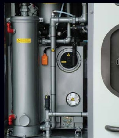
Incorporated Recuper (carbon absorber)
